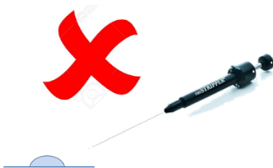
A. Horizontal pipette. It results in droplets of bigger volume and the shape is not spherical.
