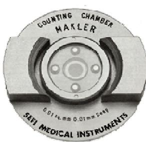
The Makler counting Chamber is only 10 µm deep and is constructed from two pieces of optically flat glass.
