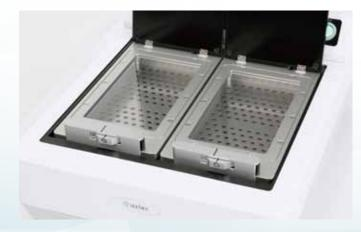
Thermal environment is optimally sheltered with a heated top and bottom of the chamber. An Observation window inherited from the EC6S model is incorporated in the Mini for a "non-disturbed" culture environment.
