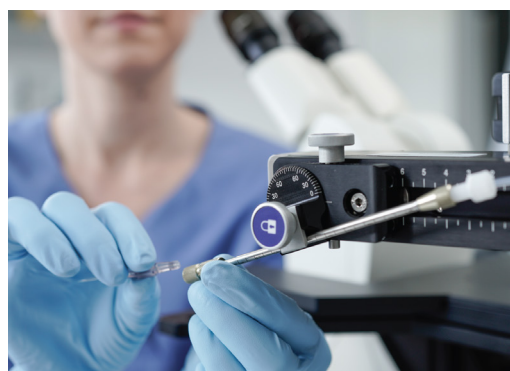
Swivel out function for easy capillary exchange.
