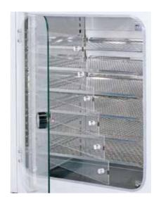
Optional shelf doors minimize the drastic change in the environment inside the chamber and reduce the amount of gas consumption and the risk of contamination.
